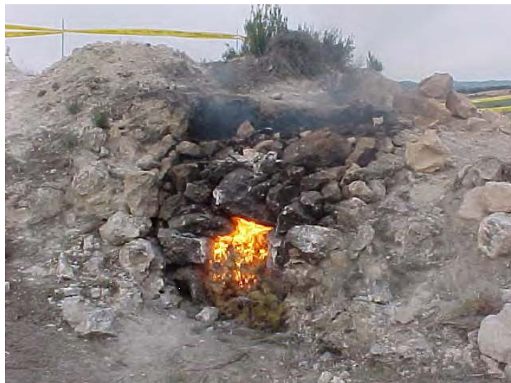
Figure 1. Handmade gypsum furnace. In Aguaviva (Teruel, Spain) [8].
