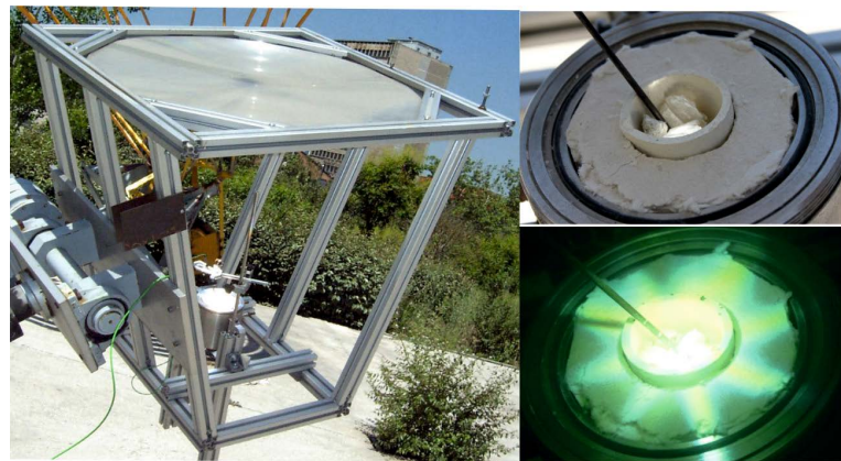
Figure 4. Solar energy concentrator (Fresnel lens). Detail of the sample chamber (before (upper right) and during solar exposure (lower right)) and the positioned thermocouple.
