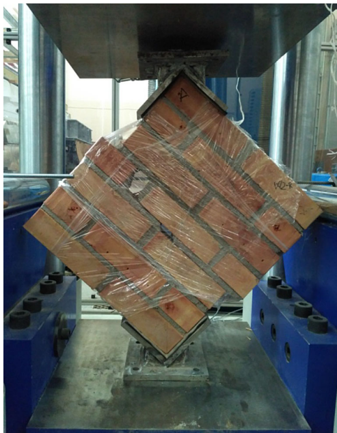
Fig. 5 Diagonal compression test: failure mode ND
