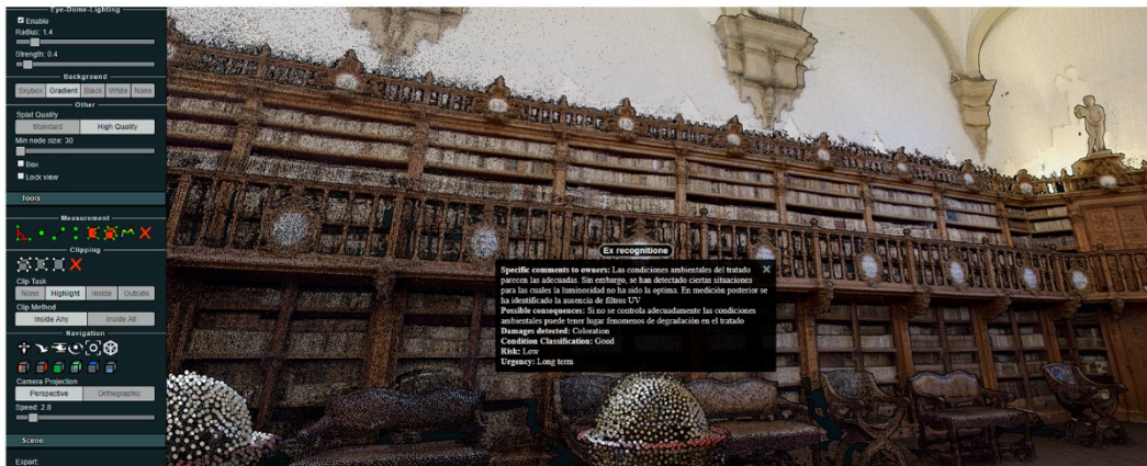
Figure 20: Non-expert user environment: a) consulting information about the asset condition; b) pop-up box related to the asset hotspot (yellow paragraphs indicate that the environmental conditions are not appropriate for the selected asset); c) 3D model
