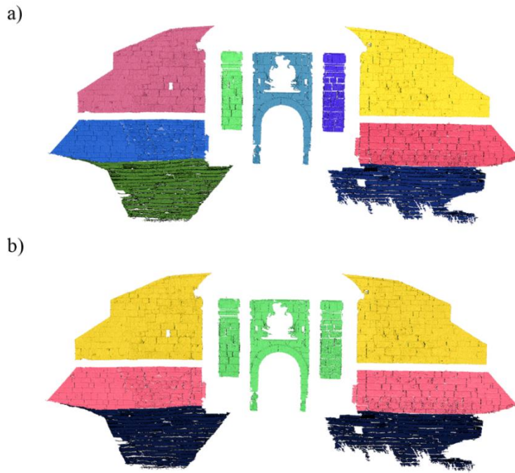
436 437 Figure 16: Segmentation carried out on façade B: (a) clusters obtained through the RANSCAC shape detector; (b) 438 planes clustered according with their similarity.
