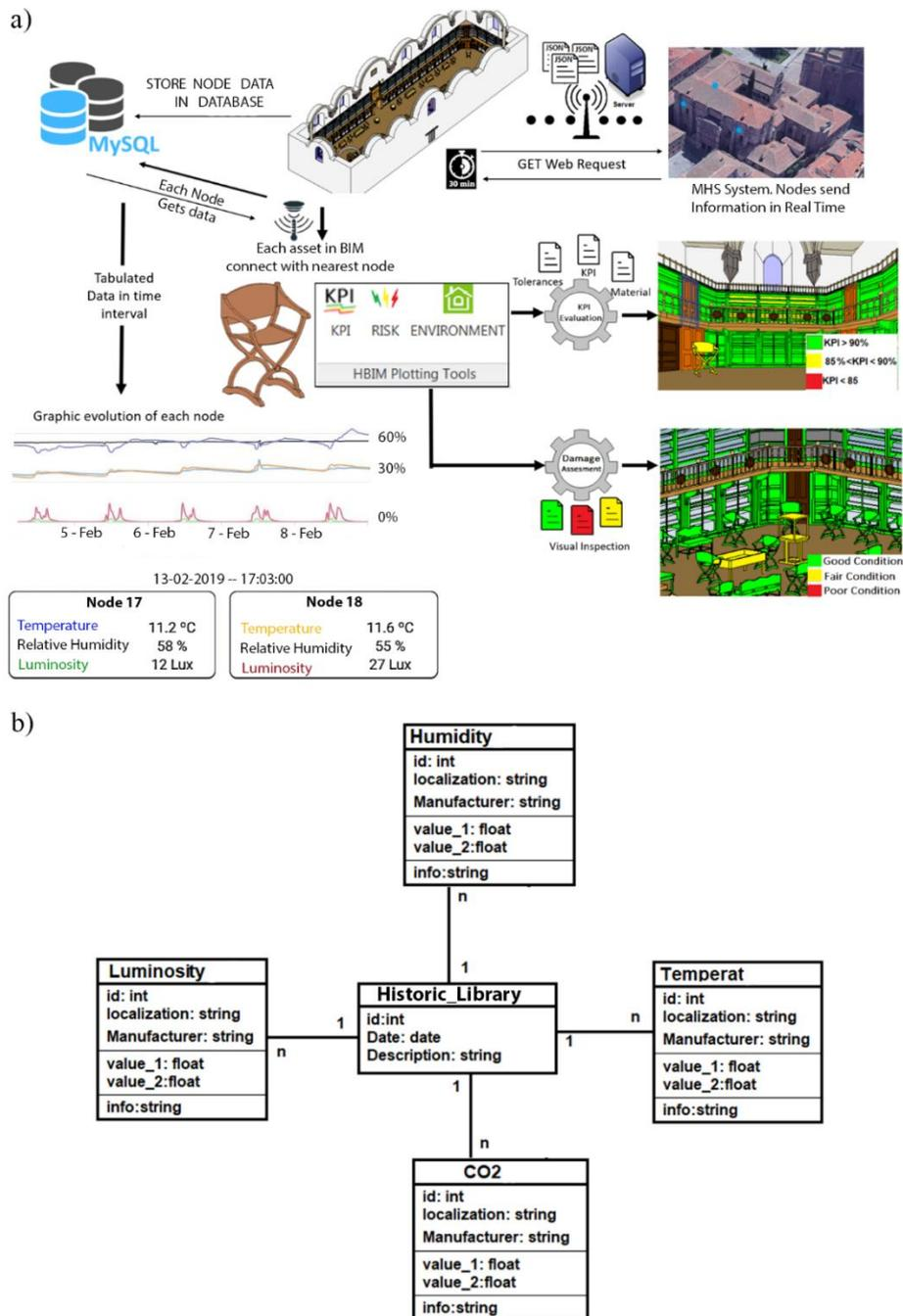
Figure 9. Connection of the monitoring network with the HBIM environment: a) general workflow;
