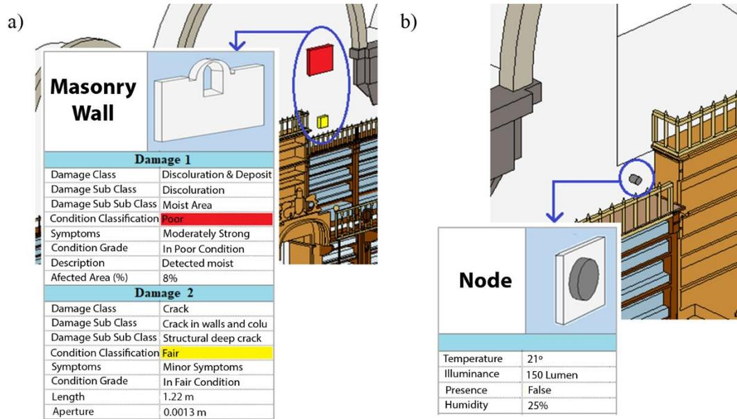
Figure 6. Damage and node objects within the HBIM model. a) Two damages with different risk attached in a construction element. b) Node patch placed in the library and its parameters
