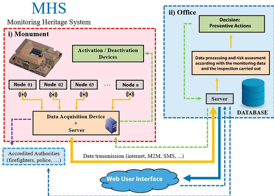
Figure 3. Scheme of the monitoring network implemented.
